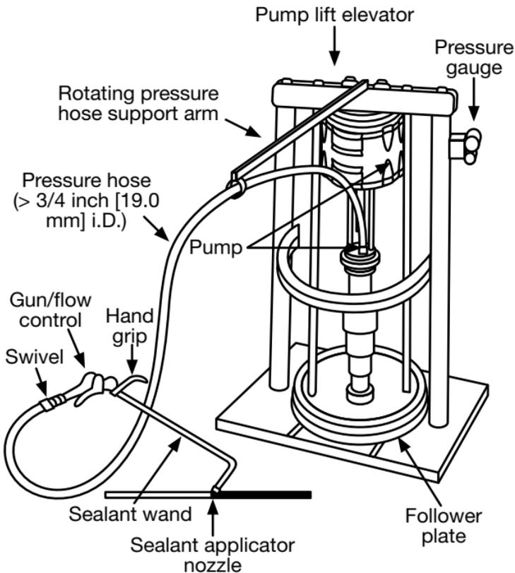
Air-powered equipment is available with varying output capacities. The ratio of the extrusion pump and accessory components of the system, especially hose diameter, will determine output volume. Specific ratios vary among manufacturers, but a ratio of 35:1 is the minimum capable of delivering a sufficient volume of sealant for efficient operation. Selection of the pump and accessory equipment should be based on desired production rates.
